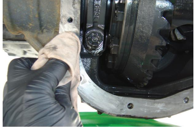
7. IF YOUR DIFFERENTIAL HAS A REUSABLE GASKET, carefully remove, clean, and inspect it for usability.
