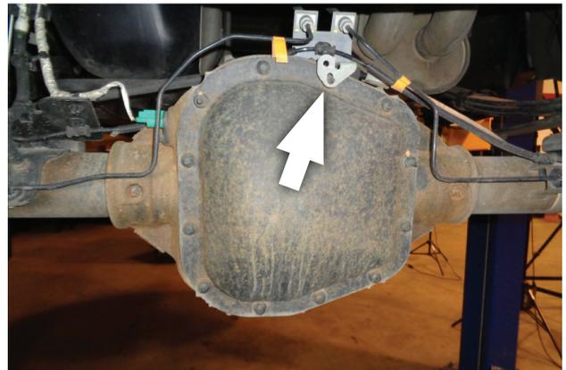
**NOTE:** On some vehicles, access to the cover may be made easier by loosening / removing surrounding parts (sway bar, brake line bracket, Panhard rod, etc.).
