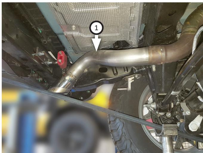
7. Fit (x2) **hanger keepers (8)** onto hanger.
