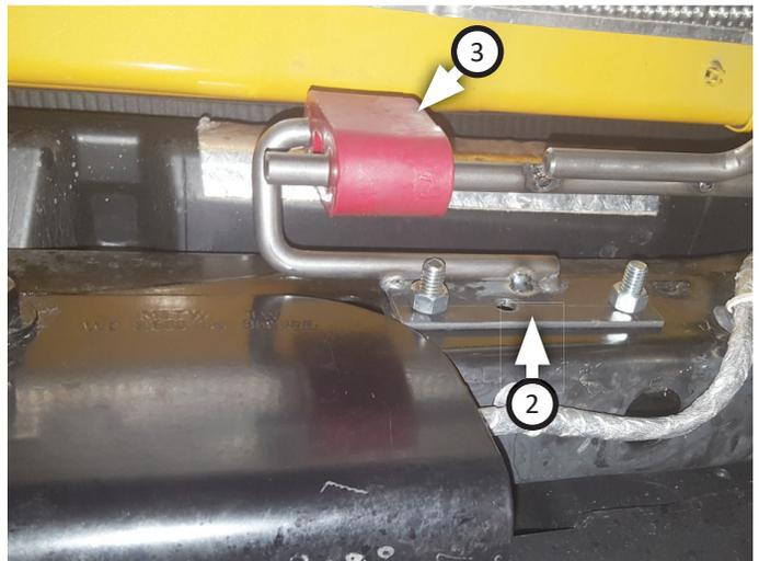
6. Connect **high exit pipe (1)** to mid pipe, inserting wire hanger into rubber hanger. Adjust muffler to fit properly as shown then tighten clamp.
