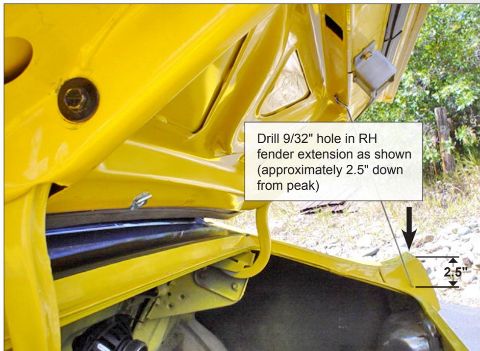
Drill 9/32" hole in RH fender extension as shown (approximately 2.5" down from peak)
