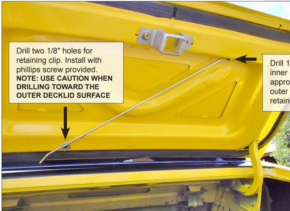
Drill two 1/8" holes for retaining clip. Install with phillips screw provided. **NOTE: USE CAUTION WHEN DRILLING TOWARD THE OUTER DECKLID SURFACE**
