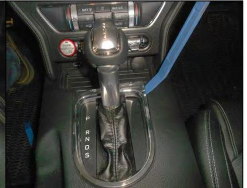
2. Starting from the front of the shift indicator, pry up to release the forward locking clips. Then work your way down the side to release the remaining ones.
