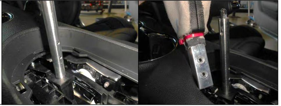
11. With the shift boot still inverted slide the Hurst pistol grip down over the lower stick and secure it in place using the two provided set screws.
